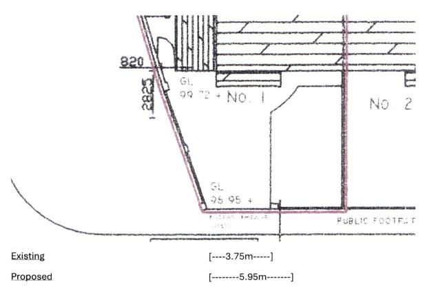
Current vehicle access width - pillar to pillar is 3.75m. This includes pedestrian access.
